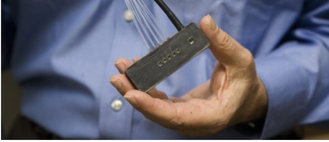
Figure 3. An fNIRS sensor that contains five light sources (only four were used) and one detector.
