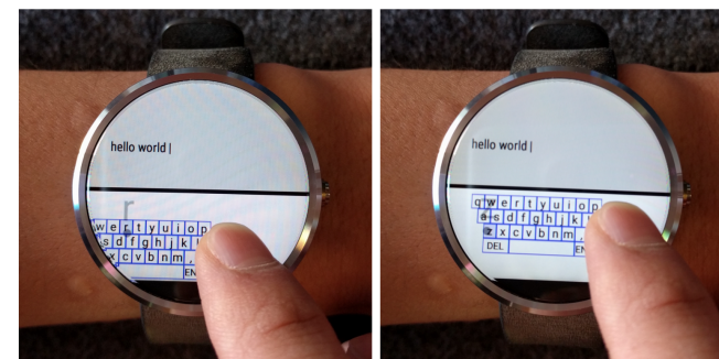
Figure 4: DriftBoard prototype in action on a smartwatch of a round display (Motorola Moto 360). Left) The fixed cursor is on top of “r”. Right) The location of the fixed cursor remains the same, but it acquires “z” as the result of the keyboard move. Note that in the DriftBoard concept, the size of the movable keyboard does not necessary to be the same as the device’ frame size. Note also that DriftBoard is applicable to more shapes than just a rectangle.
