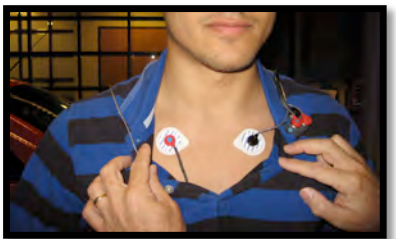
Figure 2. SCL sensor (top) and ECG sensors (middle, bottom) were applied before participants entered the vehicle.
